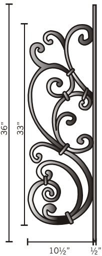
Balcony Level Rail L/H TU A1
